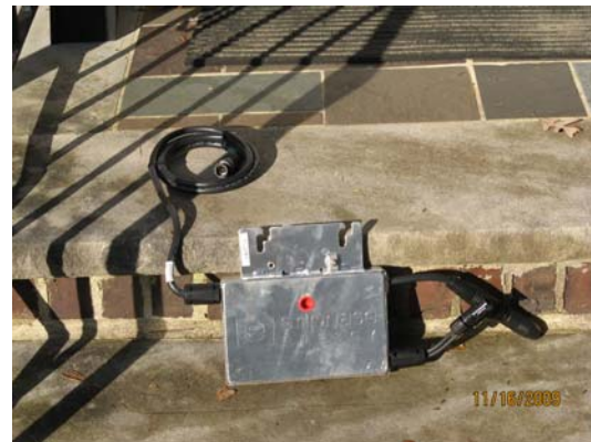
Figure 2: An Enphase M190-72 240 V microinverter that is connected to each PV module.
